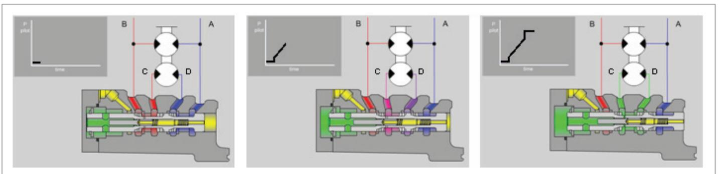
When a pilot pressure is applied to the **X** port of the motor, the main spool starts to move over its metering notches. During this period, the motor is accelerated until full pump flow passes through the **A-B** half of the motor. The **C-D** half of the motor re-circulates the flow. The inner spool then opens giving a flow path from **X** port to the idling half motor
