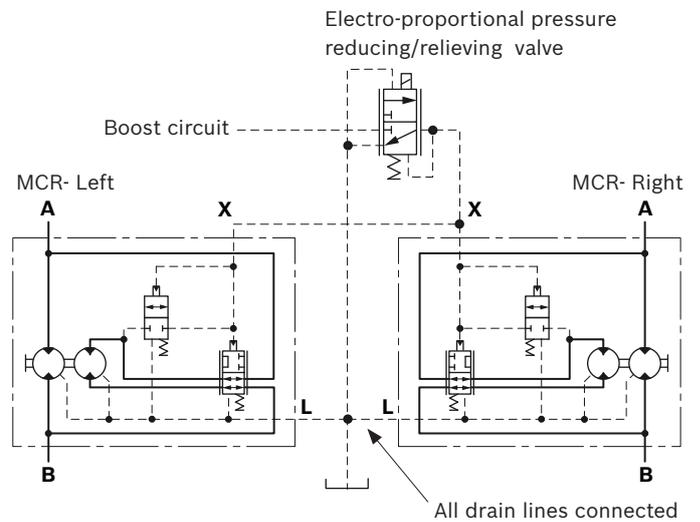
The electronic control valve can be used on vehicles that have electronic control on board. The electro-proportional pressure reducing/ relieving valve can be infinitely adjusted across a prescribed range using a solenoid input. The pressure output is proportional to the DC current input. In this way the ramp time can be proportionally controlled and adapted individually for ramp-up and ramp-down to suit vehicle dynamics as required.
