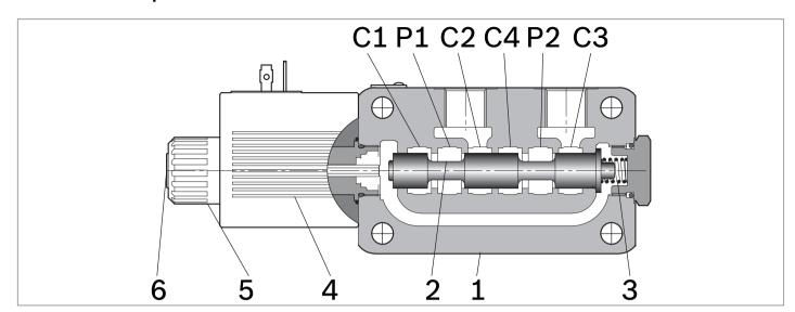
A valve basically consists of a housing (1), a control spool (2), a return spring (3) and a solenoid (5). It is designed to connect two inlet lines P1 - P2 (normally a set of hoses) and divert them to either the outlet ports (C1 - C4) with spool in position "0", when the solenoid is de-energized, or to the outlet ports (C2 - C3) with spool in position "1", when the solenoid is energized.
