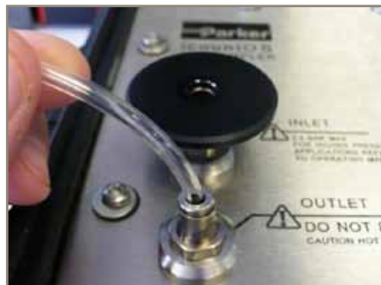
Attach OUTLET (Ø 4mm) hose
