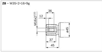
Splined shaft DIN 5480, sizes 80, 90 and 107
