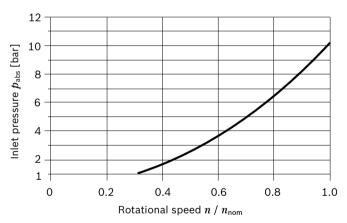
This diagram is only valid for the optimum viscosity range of  $v_{opt}$  = 36 to 16 mm<sup>2</sup>/s.
