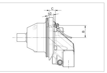
Version "M" A2FM with speed sensor DSM mounted
