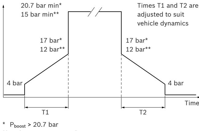
The ramp times have to be adjusted to suit the vehicle dynamics.
