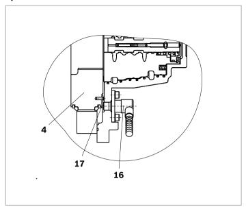
A Hall-effect speed sensor (16) may be fitted as an option, giving a two-channel output of phase-displaced square waves, and enabling detection of speed and direction. A toothed target disc (17) is fitted to the motor cylinder block (4), and the sensor, fitted to a port in the rear case, produces a pulse on each channel as each tooth passes in front of it. The frequency of the pulses is proportional to the rotational speed.
